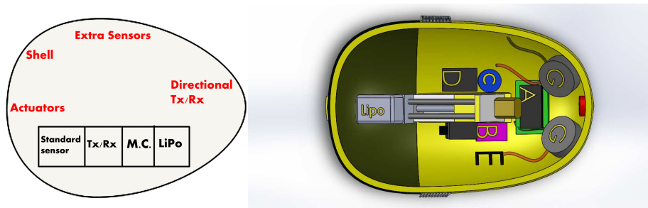
Fig. 3. Left: the additional concepts of a mobile sensor node. Right: the general design of the micro robot includes movement mechanisms that are based on linear motors, vibration actuators and dynamic center of mass.
