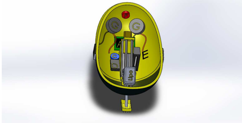
Fig. 7. Orientation change: the vibration motors (G) are used for the main rotation, while the Lipo position affects the center of mass and therefore allows controlled vertical rotation.
