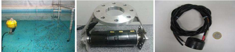
Fig. 6. Experimental setup (left), emitter (middle) and receiver (right) transducers.
