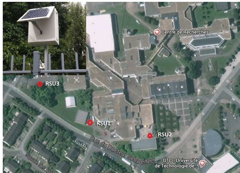
Fig. 4. Geographical position of the road-side units, RSU3 is shown in the upper left corner encased with an energy harvesting module
